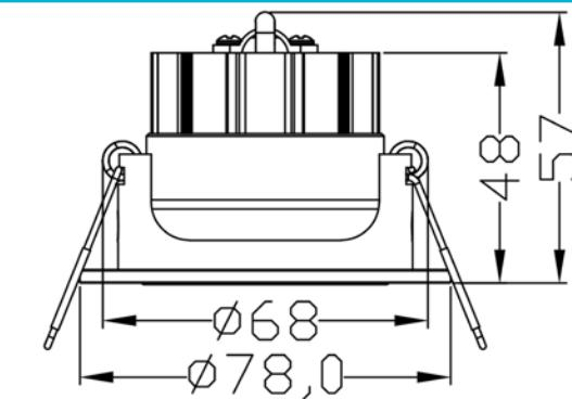
The COB 68 RGBW recessed ceiling light features our RGBW chip [RGB + warm white] developed in house, which guarantees an homogeneous colour mix in combination with the integrated reflector and enables different lighting moods using various lighting control options. The interior lights therefore are suitable both for use in living rooms and also in bars, clubs and other areas that need flexible lighting.
