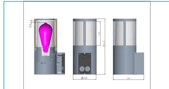
The FACADO wall light is our flexible solution for outdoor lighting. Two cable entry points allow for problem-free feed-through wiring. The removable mounting plate with plug connection and the screwless connecting terminals allow for quick and easy installation. The newly designed lamp head provides even better illumination. IP65 degree of protection ensures impressive weather resistance.
