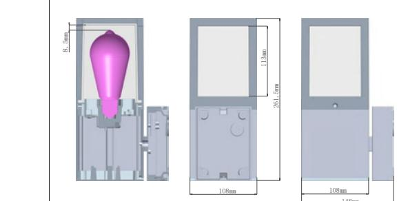
The FACADO wall light is our flexible solution for outdoor lighting. Two cable entry points allow for easy feed-through wiring. The removable mounting plate with plug connector and the screwless connecting terminals allow for quick and easy installation. The newly designed lamp head provides significantly improved illumination. IP65 degree of protection ensures impressive weather resistance.
