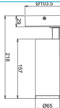
LUCEA series rotating and swivelling ceiling lights are available with 6, 10, 15, 20 and 30 W output. The lights can be customised with a rotation angle of 350° and a swivel angle of 90°. They provide up to 2,900 lumens of light output depending on the design. The light emission angle can be narrowed or expanded by exchanging optionally available lenses.
