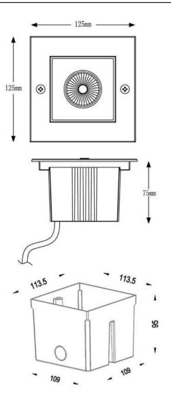
Built in ground lamp, Square COB I WW, silver, 220-240V AC/50-60Hz, 6,00 W, warmwhite
